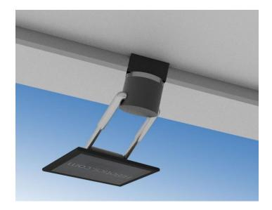
The system includes track, switcher, power system, car with 10" smart tablet, stereo speakers, microphone array, software, tracking system, and voice control.
